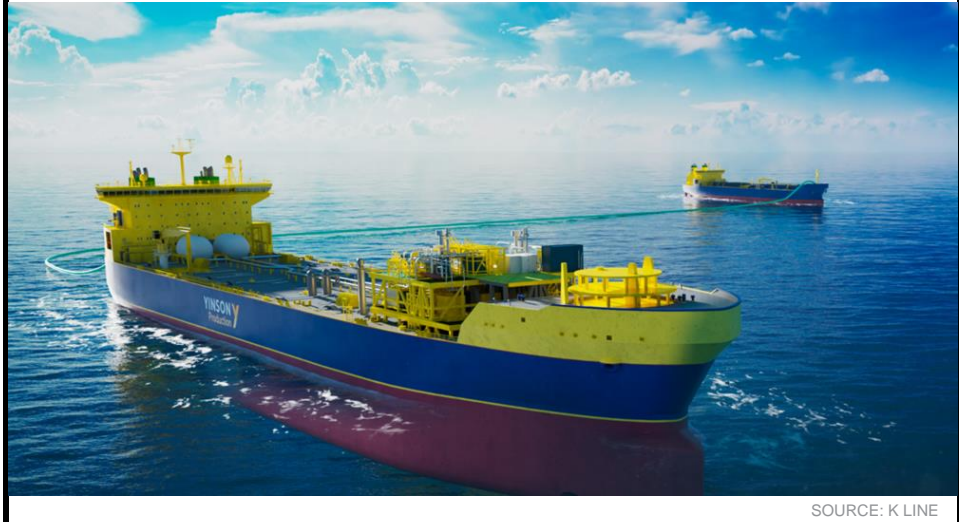
Figure 66: An illustration of an FSIU (in the foreground) receiving cargo from an LCO2 carrier (in the background)
