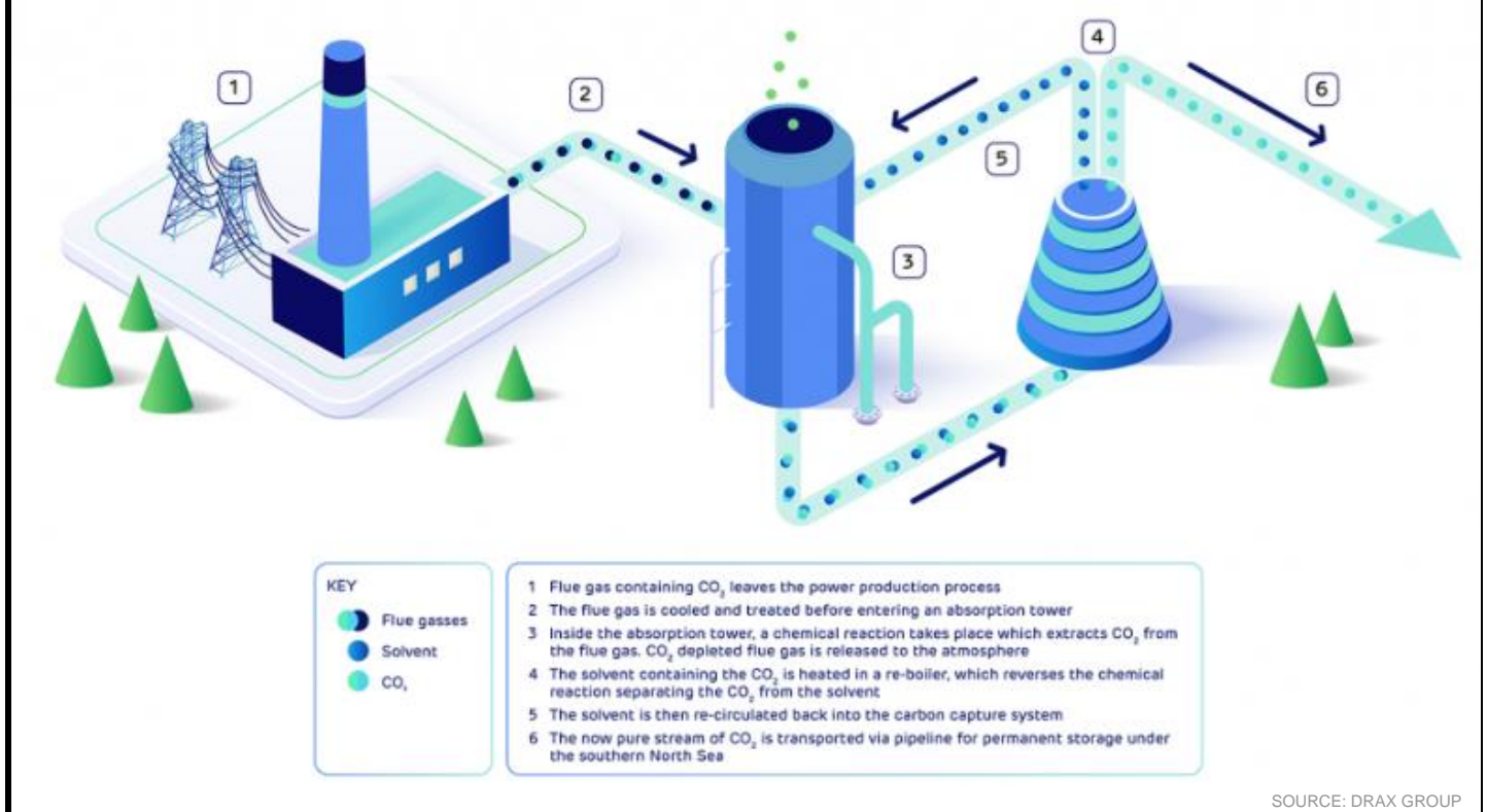
Figure 89: Illustration of BECCS, from Drax Group, which plans to make a final investment decision in 2027F to convert an existing power plant in Selby, UK, into BECCS power plant
