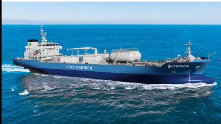
Figure 58: HD Hyundai Heavy Industries' 22,000 cbm LCO2 carrier, built for Capital Gas Ship Management
